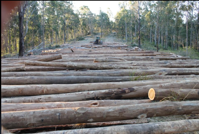
Graded commercial power poles (Spotted Gum) for Qld. NT and Asian markets (longest pole length 17.5 metres)
